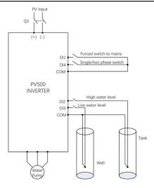
Figure 3-3 Standard wiring diagram
